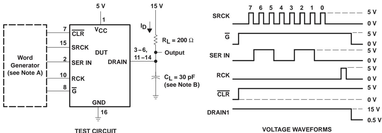
NOTES: A. The word generator has the following characteristics:  $t_r \leq 10\text{ ns}$ ,  $t_f \leq 10\text{ ns}$ ,  $t_w = 300\text{ ns}$ , pulsed repetition rate (PRR) = 5 kHz,  $Z_O = 50\ \Omega$ .
